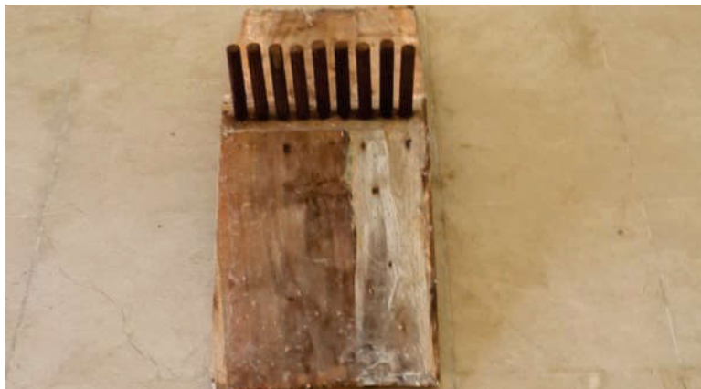
Fig. 4. Vegetation elements installed over the weir crest
