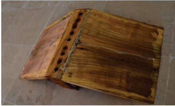
Fig. 3. Holes for installing vegetation elements
