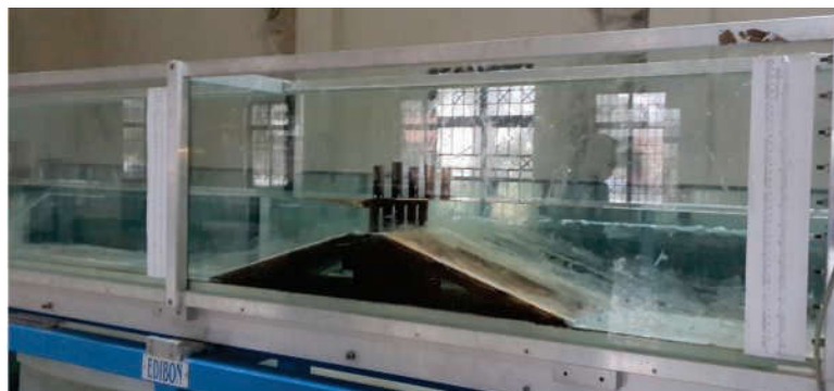
Fig. 5. Channel flow with partially submerged vegetation
